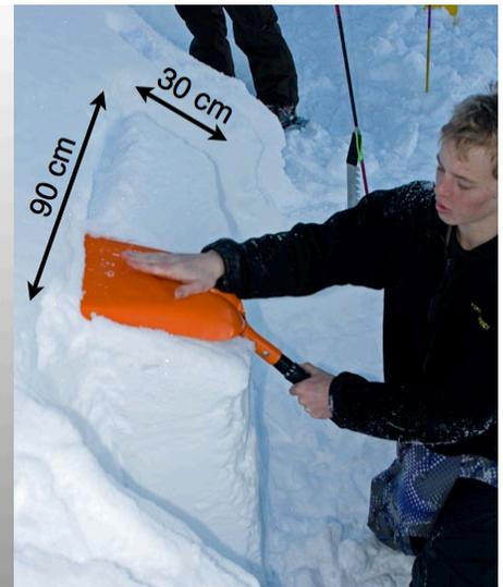
*Propagation Saw Test*, new standard test in 2009.
